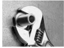
Refit the backnut and tighten with a spanner. The valve body\*\* can be held in place with a spanner, multi-grips or equivalent.
