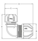
UTC® seals on a wide range of water service pipes and connects to hard and soft materials.
