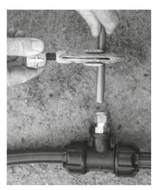
I. Cut Pipe Square Cut pipe square. Ensure the pipe is free from sharp burrs. Chamfering or lubrication is not required.
