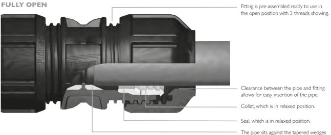
The pipe sits against the tapered wedges which minimises pipe rotation.
