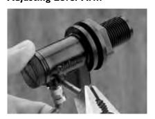
I. Where necessary bend the lever arm to adjust the water level. This can be done by removing the lever arm assembly by first straightening the tabs on the end of the pivot pin with a pair of pliers then slide it out.
