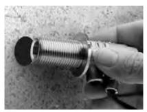
Remove the backnut and slide the thread through the appropriate sized hole.
