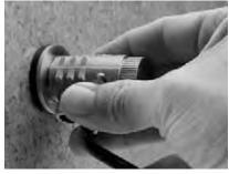
2. Where using the stem sleeve to fit the valve into 34" holes, ensure it is properly located on the valve side of the installation to prevent the valve moving.
