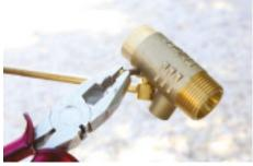
Where necessary bend the lever arm to adjust the water level. By removing the lever arm assembly and straightening the tabs on the end of the pivot pin with a pair of pliers then slide it out.
