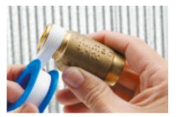
**1.** Apply PTFE tape or approved sealant to the thread ensuring a sufficient amount is applied to guarantee a watertight seal.
