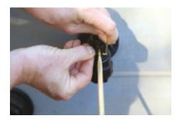
7. Replace the circlip and securethe lever.
