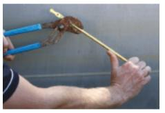
5. Using a pair of multi-grips or equivalent the lever can then bebent to the necessary angle.
