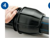
Insert the pipe up to the witness mark, or if not using a witness mark until the first point of resistance is felt.
