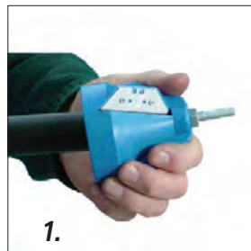
1. Cut the pipe square, then chamfer.
