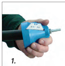
1. Cut the pipe square, then chamfer.
