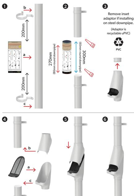
**Note:** Downpipe clip fixings not included – purchase separately to suit your cladding type. Curve is not designed for rectangular downpipe or round downpipe larger than 80mm OD. If installing Curve on 65mm uPVC downpipe extra adaptors are required. Ask your store for item code CURVE2.RA65.
