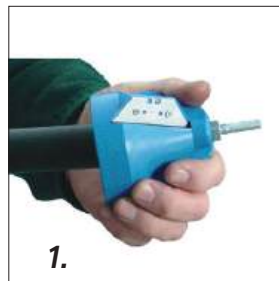
1. Cut the pipe square, then chamfer.
